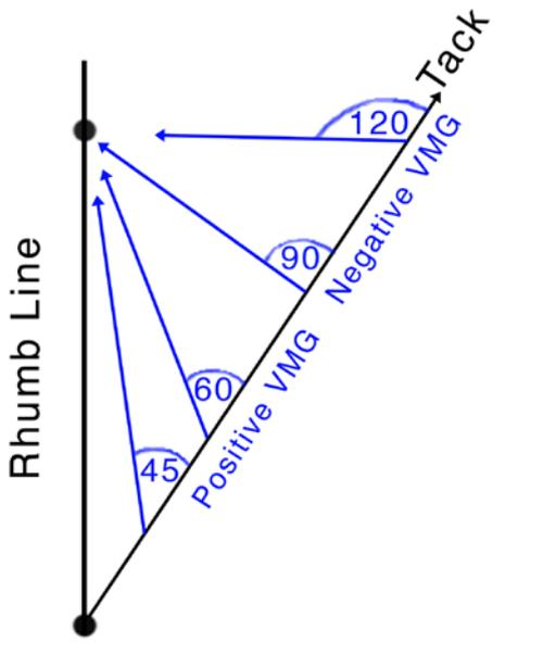
**Figure 1:** As a tack continues, the destination is increasingly off the beam of the boat at 90 degrees. As the degrees increase, you are increasingly heading away from your destination. Velocity Made Good is therefore continuously decreasing while you stay on the same tack at the same speed.
